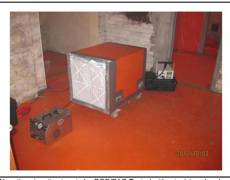
P2 Negative air unit set-up to be DOP/PAO Tested without mixing chamber.
